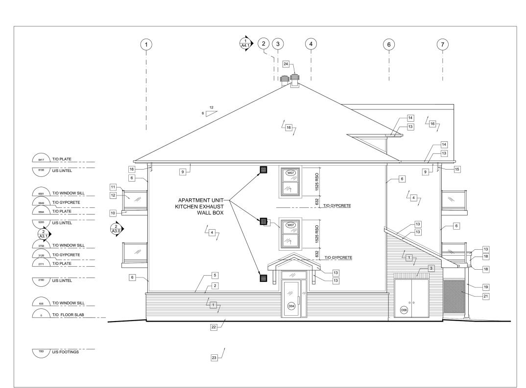
ELEVATION - NORTH SCALE: 1:100
