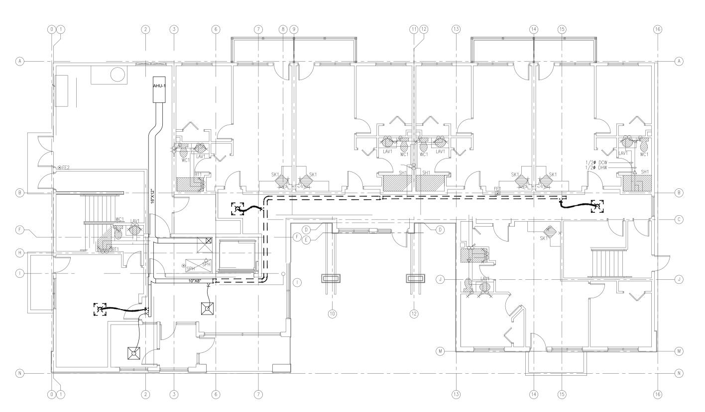
EXISTING BUILDING GROUND FLOOR PLAN - DEMO HVAC LAYOUT
